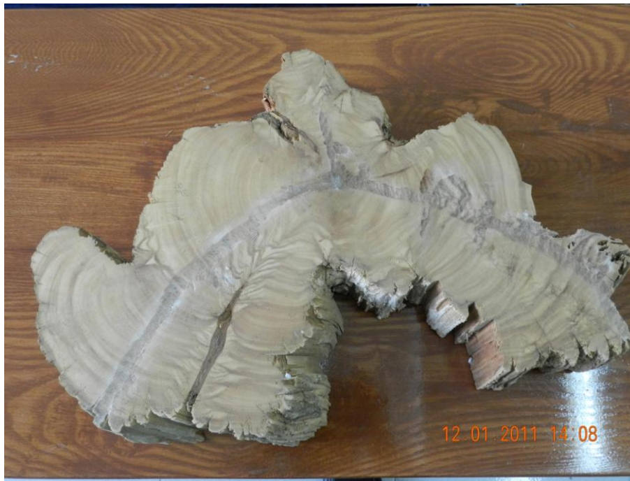
Fig. SA5. A cross section of tree MNP312. The measurement tracks can be seen as polished areas.
