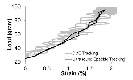
Figure S1: Load versus strain curves during biaxial testing of a porcine skin sample.
