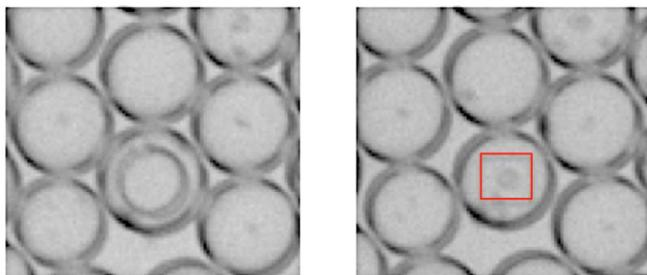
**Figure S-9.** A test system for assessing droplet stability. To identify suitable surfactant oil combinations the following test was carried out: When the type of oil surrounding aqueous droplets destabilizes double emulsions, then their formation is difficult and inner aqueous droplets combine with outer aqueous phase. As a consequence only a very small aqueous residual droplet inside an oil droplet remains behind (red square) and the format of double emulsion is lost.
