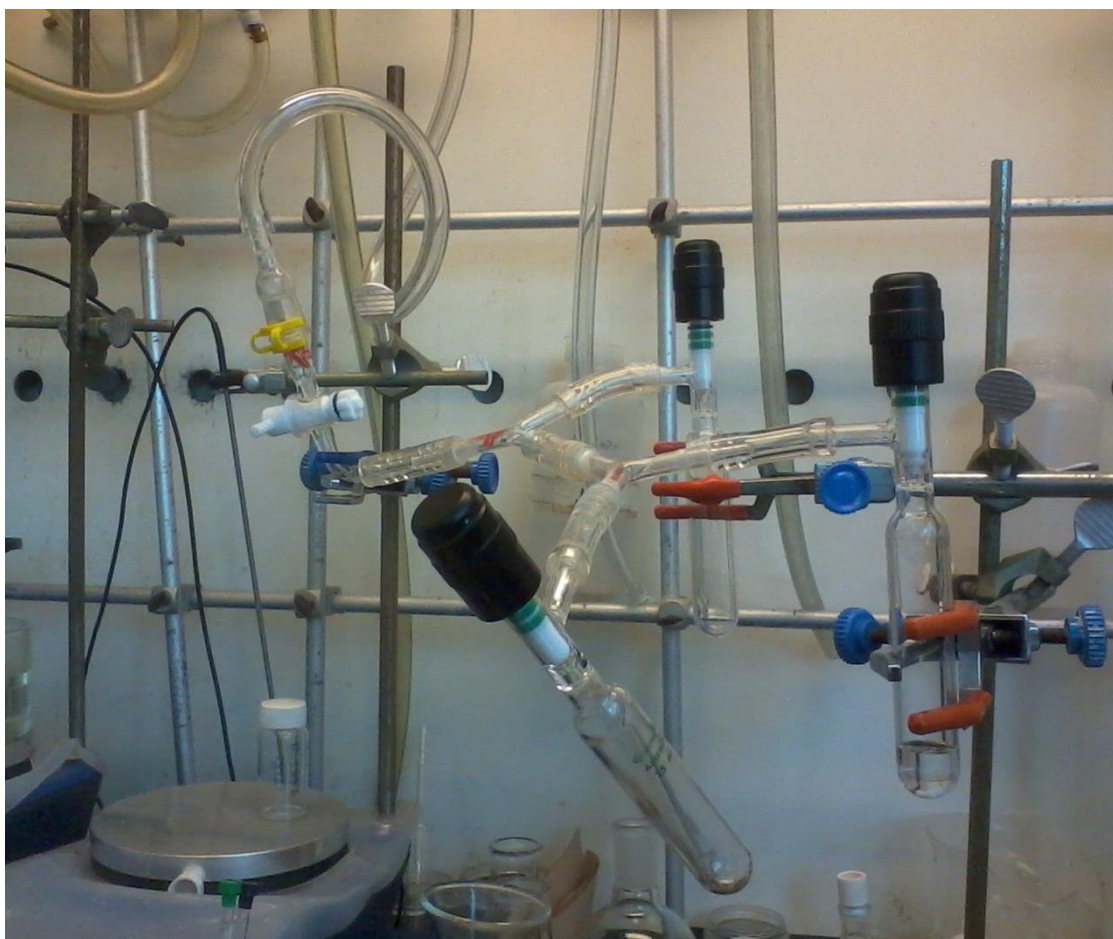
Figure S2. Apparatus for obtaining 0.29 atm.
