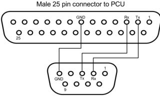
Male 9 pin connector to USB converter
