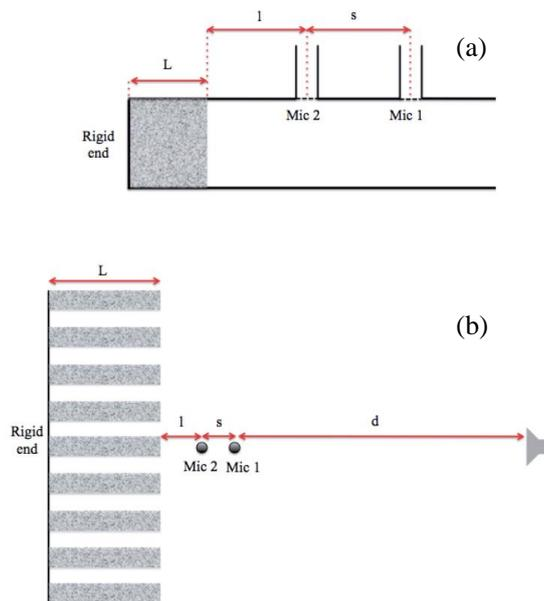
FIG. 1: Sketch for the TFM in the (a) impedance tube and (b) applied in the anechoic chamber.
