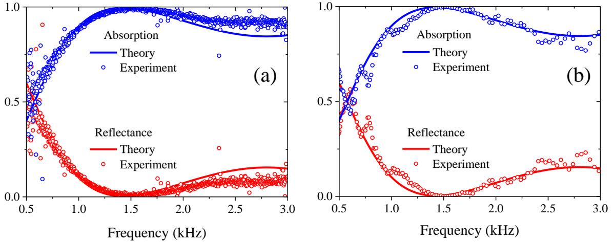
FIG. 2: Theoretical and experimental acoustic characterization of a sample of foam with length  $L = 4$  cm. We present simulations and measurements obtained by the TFM in the impedance tube (a) and in the anechoic chamber (b).
