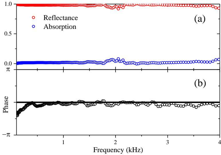
FIG. 3: Reference measurements of the rigid end. (a) Experimental data of the reflectance  $|r(\omega)|^2$  and the absorption  $A$ . (b) Theoretical (continuous line) and experimental (open circles) evaluation of the phase of the complex reflection coefficient.
