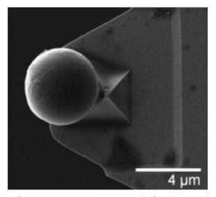
**Appendix Figure.** Scanning electron micrograph of a silica microsphere (~5  $\mu$ m) attached to the atomic force microscopy (AFM) cantilever tip after being used for adhesion measurements. Note: Protein functionalized silica microsphere remained attached to the AFM cantilever even after more than 3,000 force-distance curve acquisitions were carried out.
