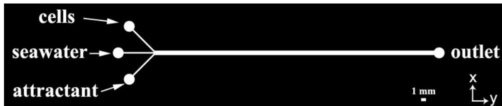
Figure S3. This 3-inlet channel is 100 \mu\text{m} deep and has three 333 \mu\text{m} wide inlets that converge to form a 1 mm wide test channel with a single outlet at the end. The three inlets are used to create parallel bands of different solutions, as indicated in the figure. Bacteria responding to the diffusive gradients of the attractant are imaged immediately downstream of the junction between the three inlet microchannels.
