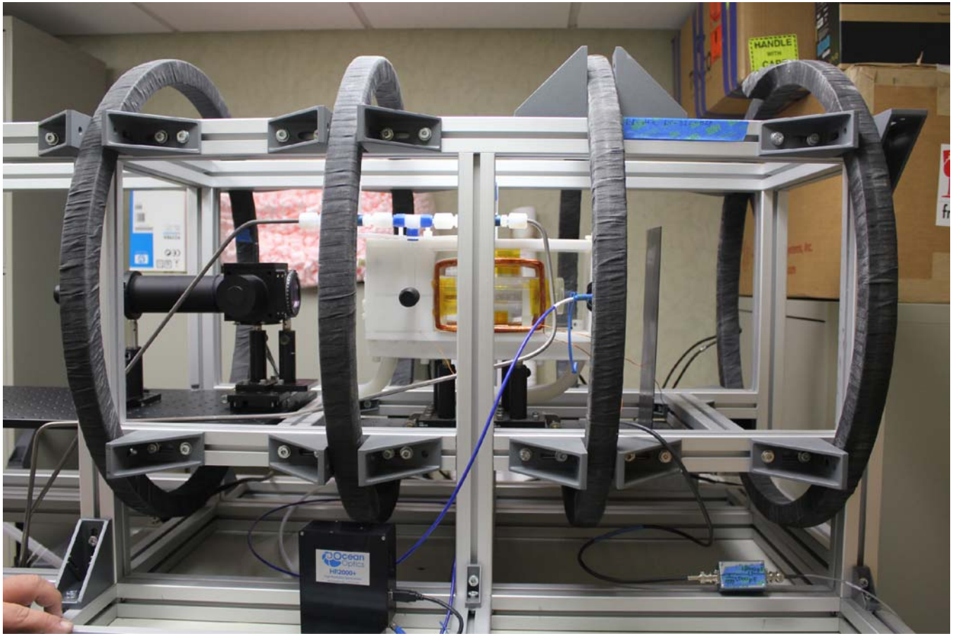
Figure S3. Corresponding photo of the right-most part of the upper frame, at a relatively early stage of polarizer construction—showing the positions of the electromagnetic coils; nominal center-to-center spacing is approximately 12 in, not including slight adjustments from shimming.
