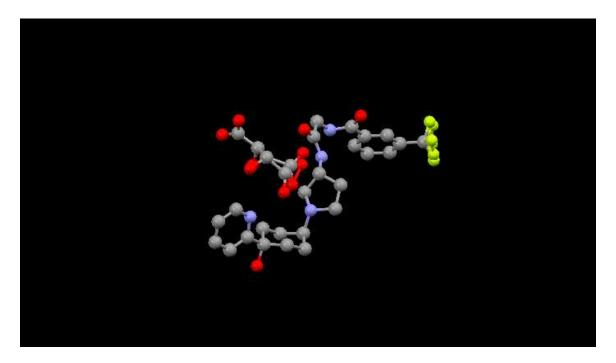
The X-ray crystal structure of the tartaric acid salt of **3** is shown with hydrogen atoms using capped sticks (top panel) and without hydrogen atoms using balls and sticks (lower panel). Grey color: carbon atoms; White color: hydrogen atoms; Blue color: nitrogen atoms; Red color: oxygen atoms; Green color: fluorine atoms.
