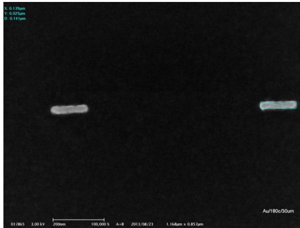
Figure S2: SEM image of gold nanorods patterned by E-beam.
