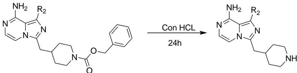
The cbz-amine is stirred in concentrated HCl for ~24 h. The reaction was then dissolved in methanol, filtered, and subjected to preparatory RP-HPLC (eluting with either a  $\text{H}_2\text{O}/\text{CH}_3\text{CN}$  or  $\text{H}_2\text{O}/\text{MeOH}$  gradient (+0.05% TFA)). After purification, the product was re-concentrated from 1.25 M HCl in EtOH to afford the final, purified product as a bis-HCl salt.
