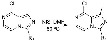
N-iodosuccinimide was added to an R<sub>1</sub>-substituted 8-chloroimidazo[1,5-a]pyrazine in DMF. The reaction mixture was heated for 5-8 h until completion (monitored by TLC (Thin layer chromatography)). The reaction was then diluted with EtOAc, washed with water, and brine. The organic layer was dried over Na<sub>2</sub>SO<sub>4</sub>, filtered, and concentrated *in vacuo*. The crude product was then purified via flash chromatography over silica, eluting with a hexanes/EtOAc gradient.
