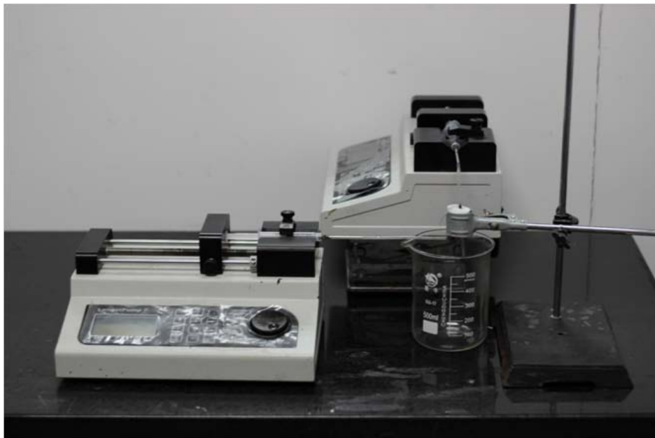
Supplementary Figure 1 Photograph of experimental apparatus for coaxial spinning.
