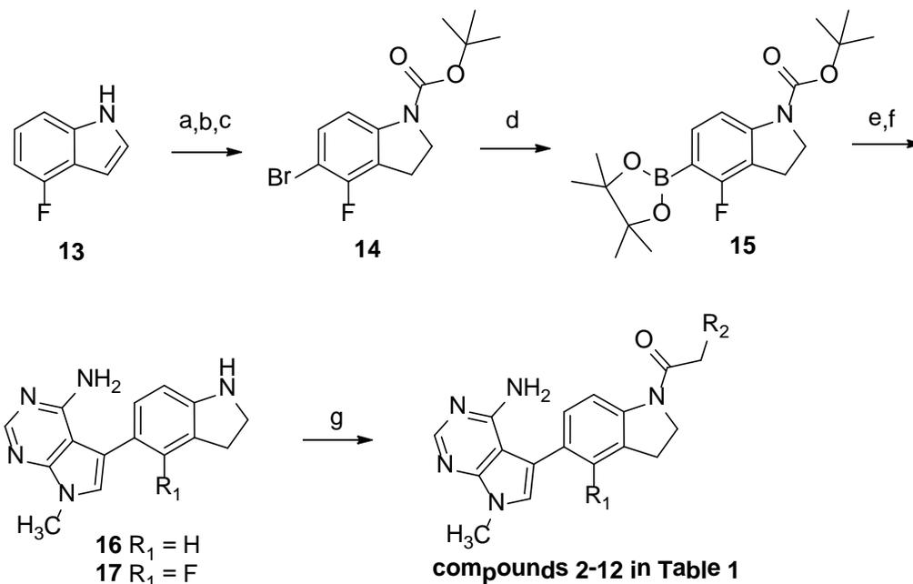
(a) NaBH<sub>3</sub>CN, HOAc, 89%; (b) Boc<sub>2</sub>O, DMAP, CH<sub>3</sub>CN, 95%; (c) NBS, DCM, 99%; (d) bis(pinacolato)diboron, KOAc, PdCl<sub>2</sub>(dppf); (e) 5-Bromo-7-methyl-7H-pyrrolo[2,3-d]pyrimidin-4-amine,<sup>1</sup> K<sub>3</sub>PO<sub>4</sub>, (t-Bu)<sub>3</sub>PHBF<sub>4</sub>, Pd<sub>2</sub>(dba)<sub>3</sub>, 80°C; (f) HCl, dioxane; (g) heteroaryl acetic acid, coupling reagent
