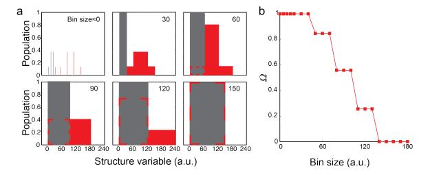
Measuring the nature and extent of similarity between ensembles using 2D  $\Omega$  versus bin size.
