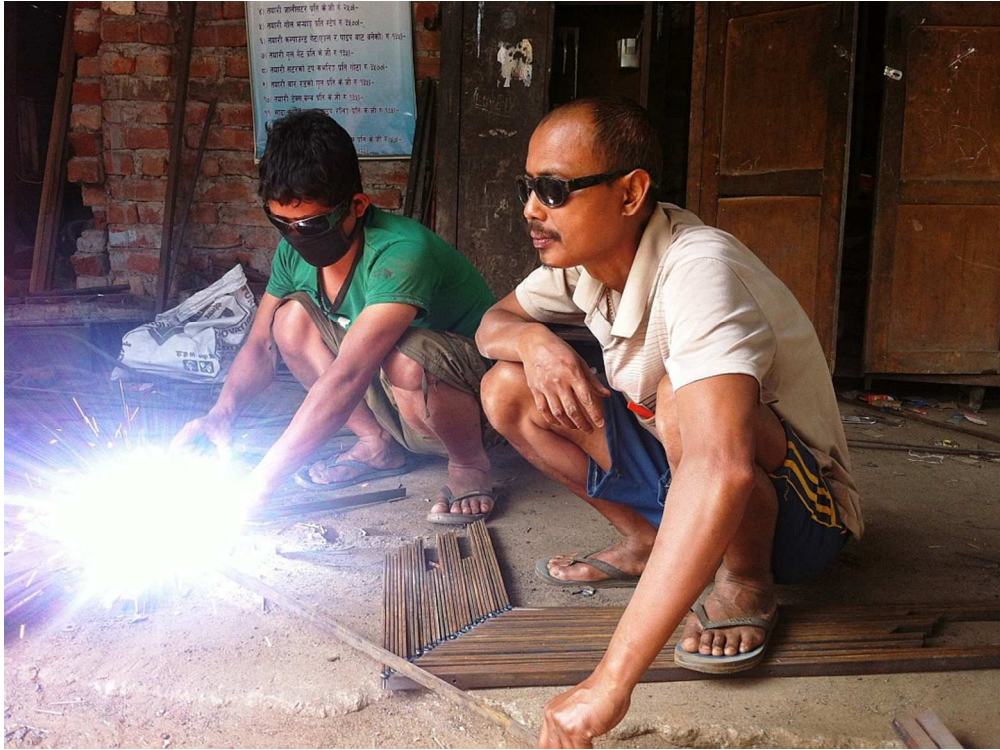
Welders at work using only sunglasses and cotton mask during welding in Nepal 90x67mm (300 x 300 DPI)
