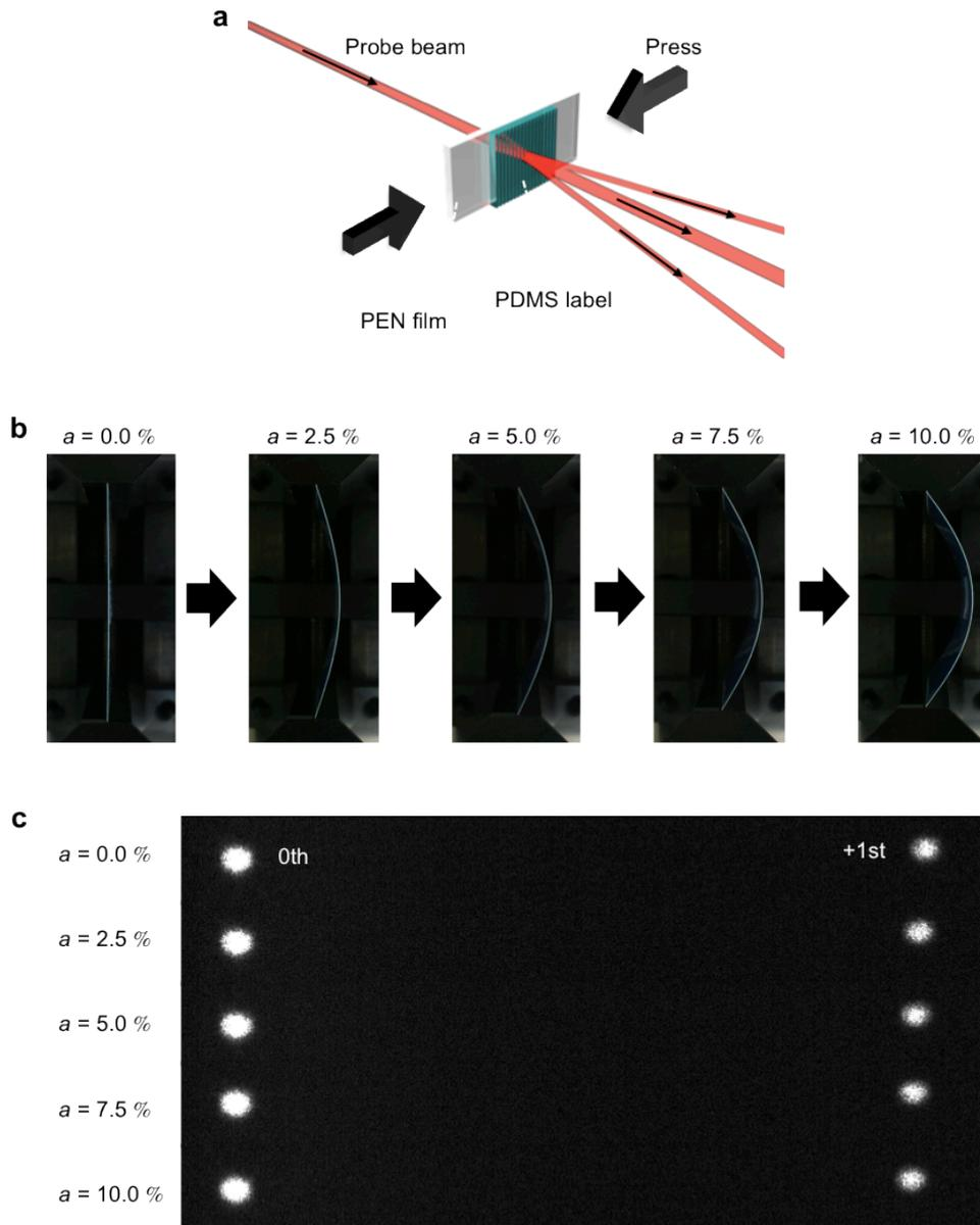
**Figure S8. Surface-strain analysis of PEN film by the surface-labelled gratings.**
