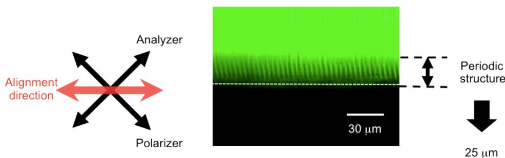
**Figure S4. Polarized optical micrograph of the cross-section of the film after the grating formation.**
