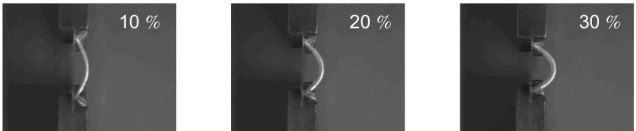
**Figure S7. Top-view of mechanically bent single-layer and bilayer PDMS films.**
