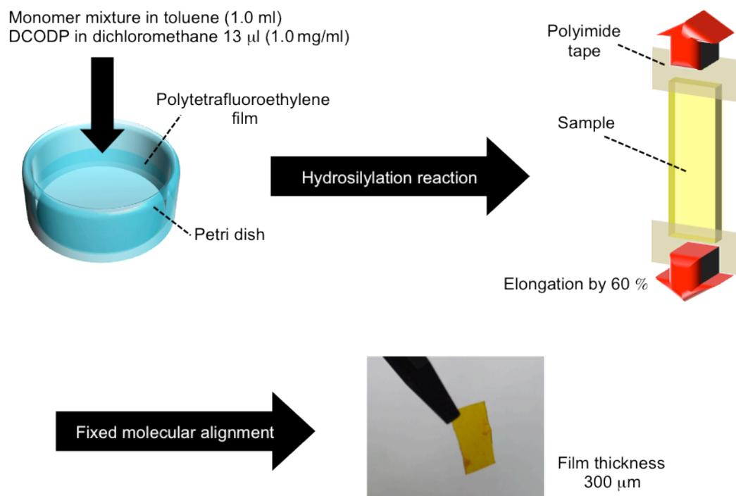
Figure S2. Preparation of azobenzene-containing liquid-crystalline elastomer films by a two-step method.
