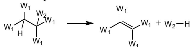
$W_1$  = C or halogen.  $W_2$  must be a halogen.
