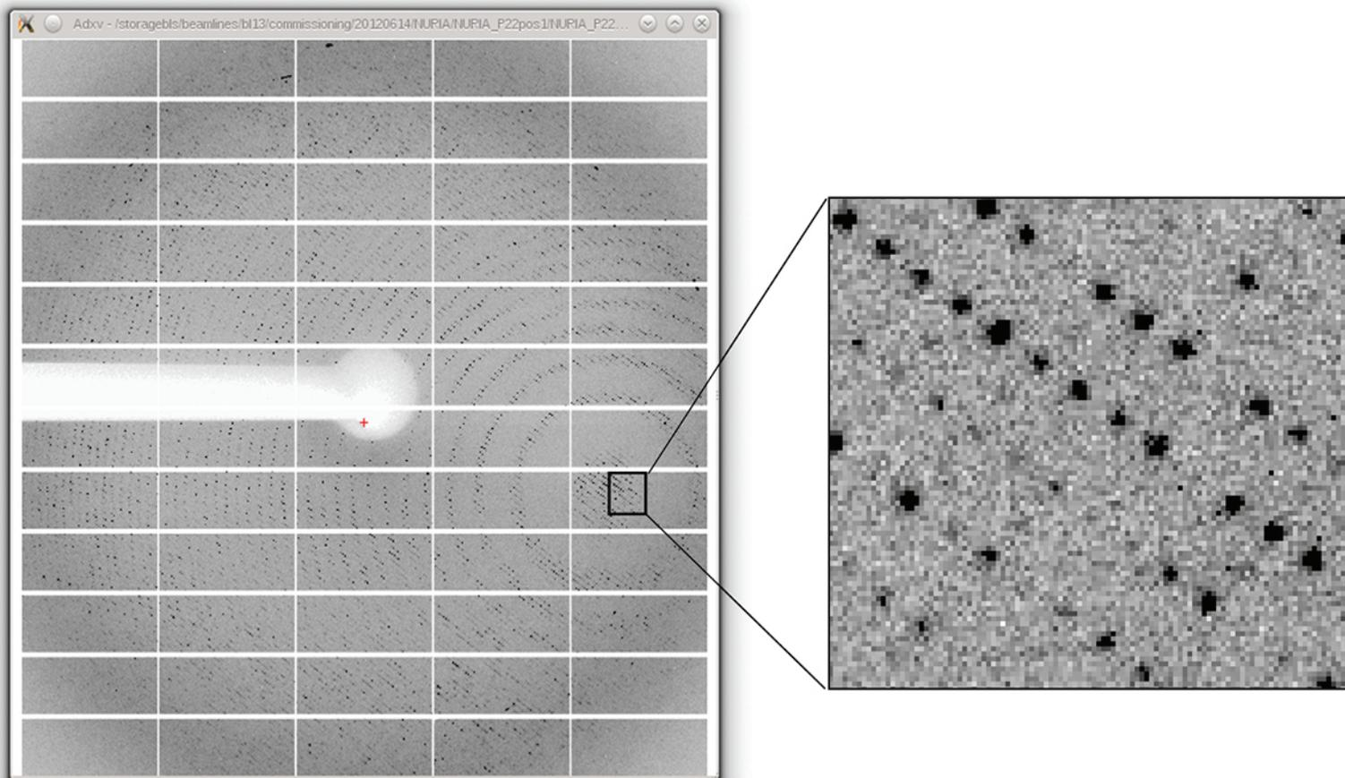
**Fig. S1** A diffraction frame from crystals of Human Rhinovirus 2 (N. Verdaguer) taken with the Pilatus 6M detector. The data collection parameters are listed in Table 2 of the paper.
