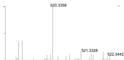
Figure S14. Retention time selected isotope envelope for LPC (18:2). A 184 head group fragment is also observed in the fragmentation spectrum below.
