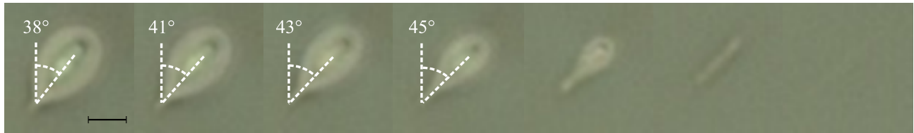
Supplementary Figure 4: Waveguide tilt achieves 45°. Microscope images of the cross sections of the waveguides fabricated with 2w = 0.75 \mu\text{m} . The black scale-bar is 5 \mu\text{m} long.
