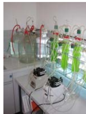
Five chemostats with peristaltic pumps in the foreground and feeding bottles in the background
