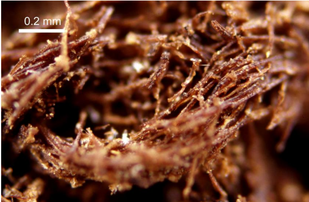
Figure S9: 33.30.83 Tomb No. 1214, Badarian Period, Mostagedda Epi-darkfield (HD) illumination. A sector stop in the light path together with a rotating stage has been used to accentuate the relief. The limited depth of field is a major disadvantage of the technique.
