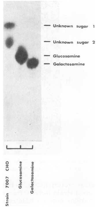
FIG. 4. Paper chromatogram showing the hydrolytic products from the 7007 antigen after hydrolysis in 2.0 N HCl at 100 C for 18 h.
