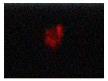
Movie S1. The alignment He-Ne after propagating the full 400-m path length. The oscillations seen in the beam are the result of scintillation and demonstrate the rapid deterioration of the beam quality of a high-quality Gaussian beam propagating over long distances.
