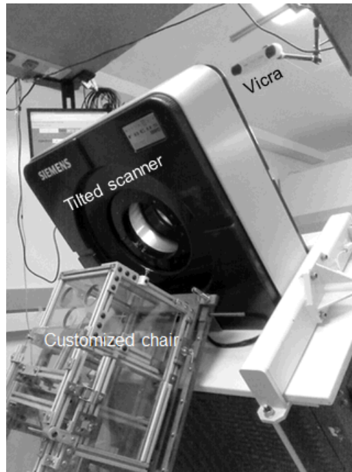
Supplemental Fig. 4. MicroPET scanner FOCUS-220 raised and tilted forward \sim 45^\circ with a lifter-tilter. The Vicra camera was hung on the ceiling and positioned towards the bore of the scanner.
