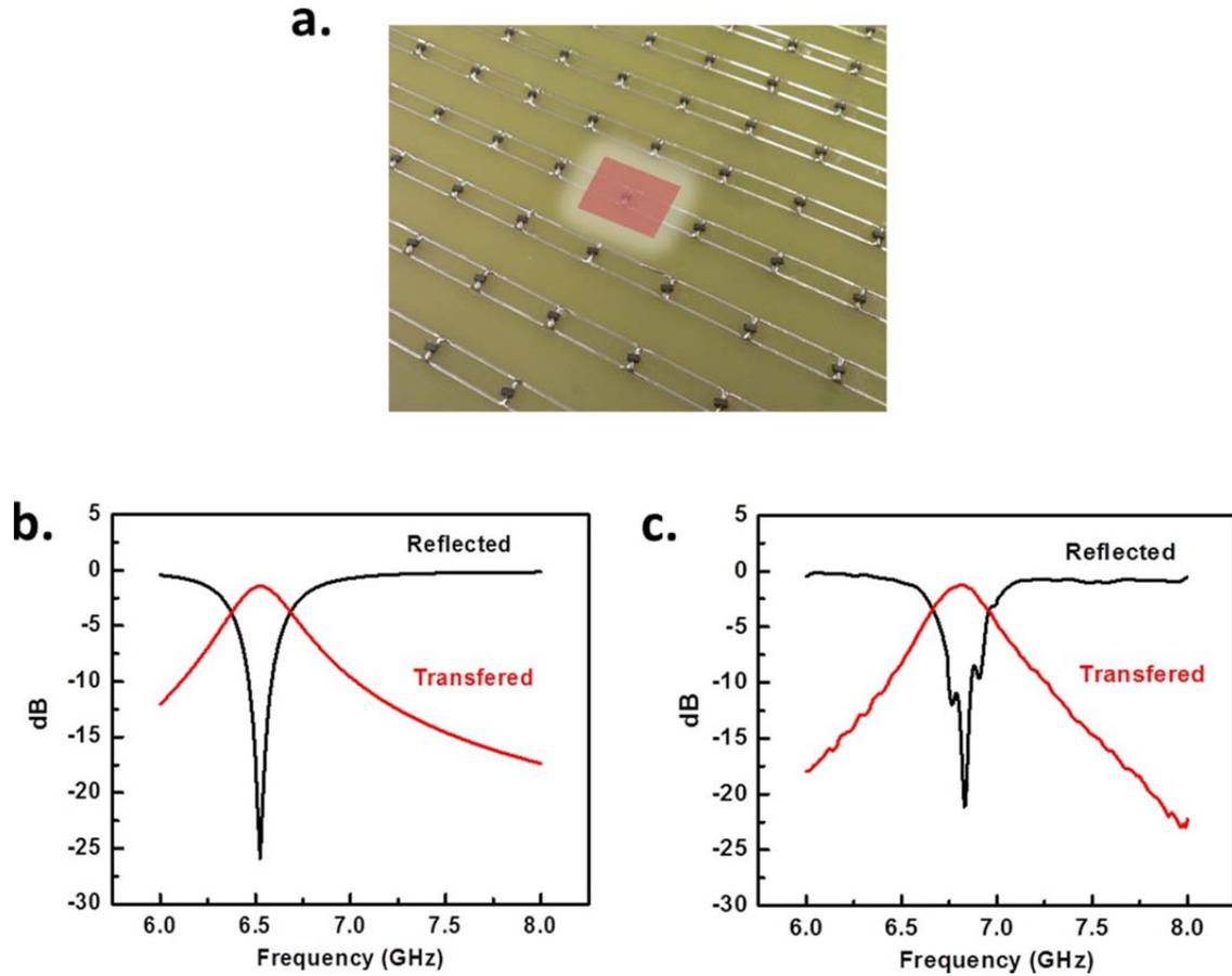
Figure.S2 (a) The picture of the UEECA constructed using FR4, the ratio of the reflected and transferred microwave in (b) simulation and (c) measurement.
