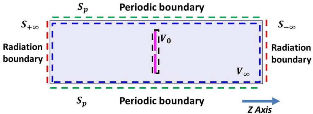
Figure.S3 A sketch of the structure with only the front structure as in Fig. 1 (a). The notations include the radiation boundary surfaces in the positive (negative) z axis  $S_{+\infty}$  ( $S_{-\infty}$ ) indicated by the red dashed lines, periodic boundary surfaces  $S_p$  shown by the green dashed lines, far field volume  $V_\infty$  surrounded by the blue dashed line, and the volume containing only the antenna  $V_0$  surrounded by the black dashed line.
