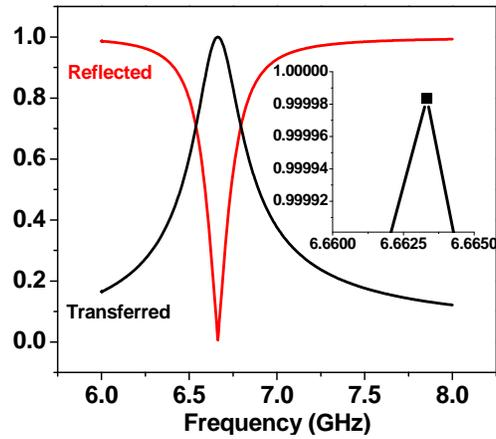
Figure S1. The Simulated S-parameters of the UEECA with zero loss material.
