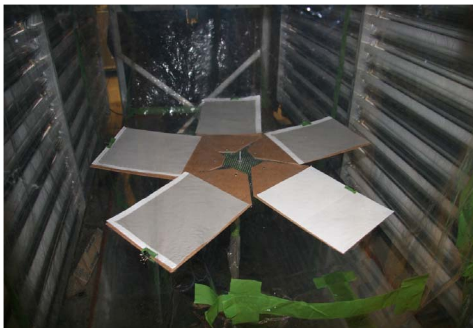
Figure S2. Apparatus used for exposing filters to \text{N}_2\text{O}_5/\text{NO}_3/\text{NO}_2 . Shown is a filter coated with deuterated PAH (that at the 5 o'clock position) and four filters on which ambient particles were collected.
