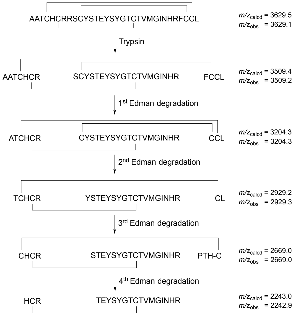
Scheme S1. Determination of disulfide bond connectivity of F2A by employing trypsin digestion and manual Edman degradation. This step-by-step summary applies for all HD6 mutants analyzed in this work. The calculated and observed masses of all mutant HD6 are listed in Table S3.
