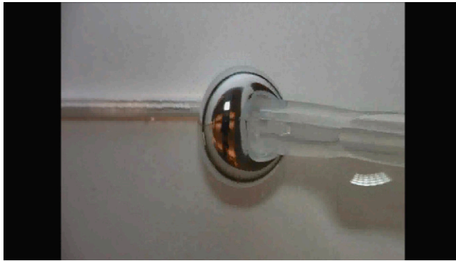
Movie S3. After mechanically distorting a droplet of the metal, it returns to an equilibrium shape.
