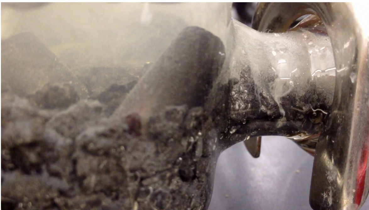
Figure S7. Screenshot of hydrogen gas evolving off of a biocathode. Video screenshot of a biocathode in phosphate buffered media poised at -600 mV vs. SHE.
