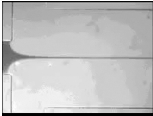
Movie S1. Performance of microfluidic control of the central stream of ATP in response to a sinusoidal reference input.
