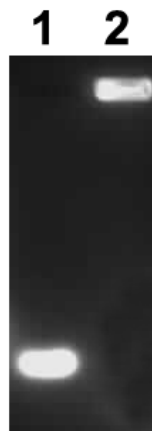
Figure S16 Agarose gel electrophoresis of naked siRNA (Lane 1) and siRNA/UiO-Cis (Lane 2) showing the siRNA loading into the NMOFs.
