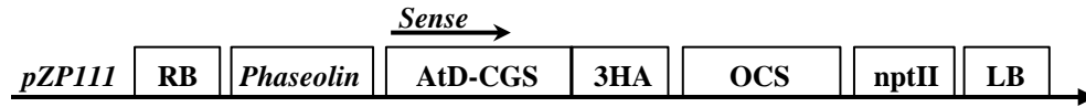
Figure S1. The plant transformation binary vector construct for seed-specific expression of AtD-CGS. The cDNA for AtD-CGS was inserted in the sense orientation under the control of the seed-specific phaseolin promoter into the binary vector pZP111 carrying three in-frame copies of hemagglutinin (3xHA) epitope tag and an octopine synthase (OCS) terminator as illustrated. The nptII gene was used as the selectable marker for kanamycin selection.
