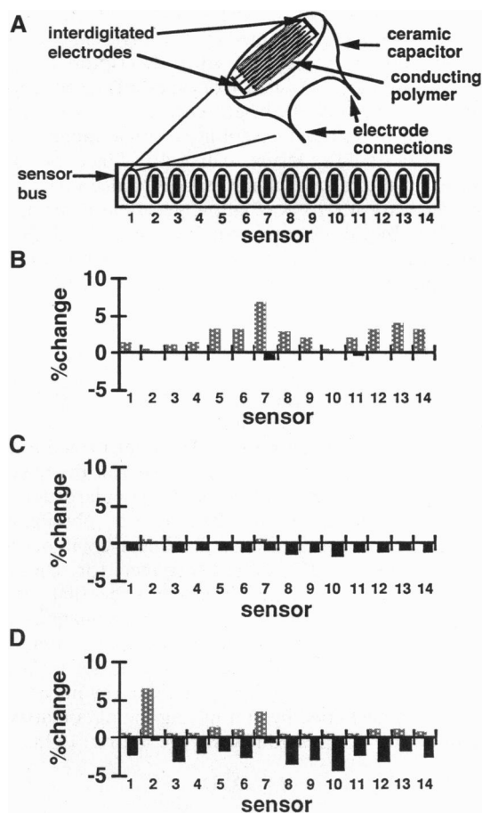
FIG. 1. (A) Schematic of a sensor array showing an enlargement of one of the modified ceramic capacitors used as sensing elements. The response patterns generated by the sensor array described in Table 1 are displayed for acetone (B), benzene (C), and ethanol (D). The sensor response was defined as the maximum percent increase and decrease of the resistance divided by the initial resistance (shaded bars and solid bars, respectively) of each sensor upon exposure to solvent vapor. In many cases, sensors exhibited reproducible increases and decreases in resistance. An exposure consisted of (i) a 60-sec rest period in which the sensors were exposed to flowing air (3.0 liters/min), (ii) a 60-sec exposure to a mixture of air (3.0 liters/min) and air that had been saturated with solvent (0.5 liters/min), and (iii) a 240-sec exposure to air (3.0 liters/min).
