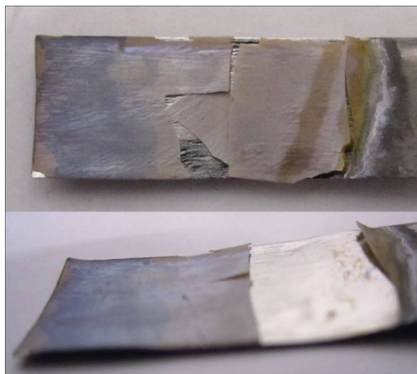
Figure S3. The influences of detachment and consolidation of different parts of the same specimens soaked in different solvents. The post-treatments by protic solvent (pure methyl alcohol, the right part stripped automatically) and aprotic solvent (pure acetone, the left part adhered on substrate tightly) can influence the adhesive strength of the tube layers to the substrate in an opposite way.
