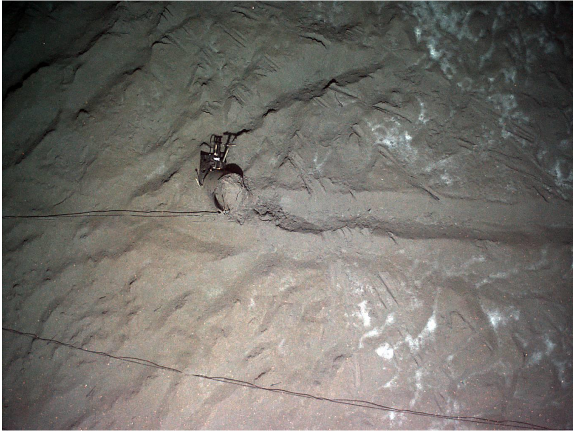
Supplementary Figure 2: Downward-looking Sentry photograph of the pH sensor. The trail runs from the sensor towards the frame. The trail is approximately 35 cm wide. Source: WHOI ABE/Sentry team.
