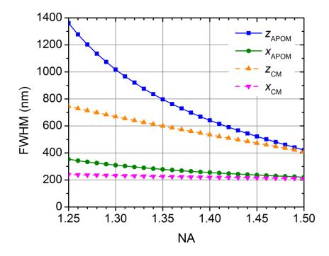
Calculated FWHM of the PSF of APOM and a conventional wide-field microscope (CM) along the x (lateral) and z (axial) axes as a function of the NA of objective lenses for the wavelength of 546 nm. Note that a CM cannot image the axial plane directly. We calculate the FWHM of the PSF of a CM for comparison only. The PSF is not symmetric along the x and z axes for both APOM and CM's. The resolution of APOM approaches that of CM for high NA objective lenses.
