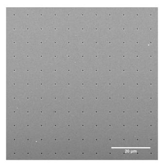
A SEM image of the nano-hole array used for calibration of the APOM. The period of the array is 7  $\mu$ m, and the diameter of each hole is 500 nm. The nano-hole array is fabricated by a focused ion beam (FIB) on a 150 nm gold film deposited on a glass coverslip. The small defects (bright spots) near the right top corner and the left bottom corner of the nano-hole array are also visible in the optical image taken by APOM (Fig. 2d in the main text).
