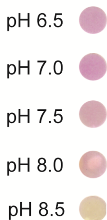
Figure S8. NP-free test strip response against pH buffered drinking water solutions at relevant pH levels.
