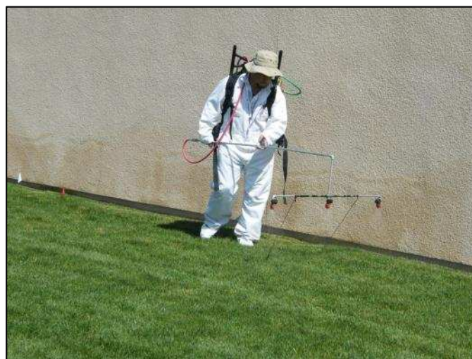
Figure S4-2. A single pass was made to achieve the grass perimeter application. A three-nozzle spray boom was used to produce the desired spray width of 5 feet.
