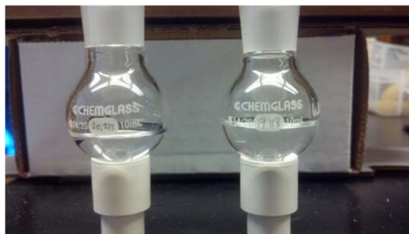
Figure S8. Showing the similar surface area of the standard reaction (0.231 mmol) and a reaction at twice the scale (0.5 mmol).
