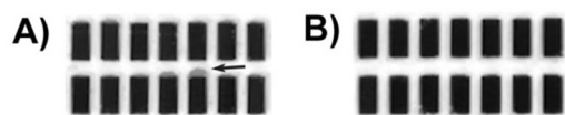
Figure S-5. Images of filled chambers at ambient pressure following sample digitization. A) When using an air compressor to drive flow during digitization, some chambers overflow and sample is pushed into the main channel after pressure is released. The arrow indicates an area where sample exits the chamber. B) When vacuum pressure was used to digitize the sample this effect was not present.
