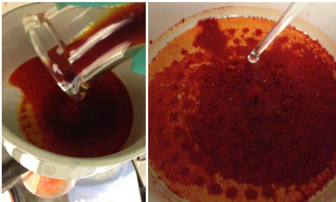
Figure S10. Collecting the recrystallized \text{Fe}(\text{dibm})_3 . From left to right: filtering through a Büchner funnel, rinsing with aqueous EtOH pre-cooled to -78\text{ }^\circ\text{C} .
