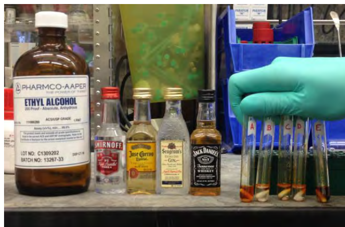
Figure S23. Reaction mixtures using solvents A–E prior to heating at 60\text{ }^\circ\text{C} .
