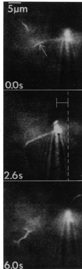
FIG. 2. Three micrographs showing an individual force measurement. (Top) At 0.0 s the actin filament, attached to the microneedle, is beginning to engage (indicated by arrow) the skeletal muscle myosin-coated surface. (Middle) After 2.6 s, force has reached steady state, and the microneedle is maximally deflected. (Bottom) At 6.0 s, the actin filament detaches from the microneedle, allowing the microneedle to return to its original position. The dashed line indicates microneedle position at zero force; the perpendicular solid line marks the extent of needle deflection, which was used to calculate force. The bright microneedle tip is due to numerous fragments of adherent fluorescently labeled actin filaments. Slight bright-field illumination improved visualization of the microneedle outline.
