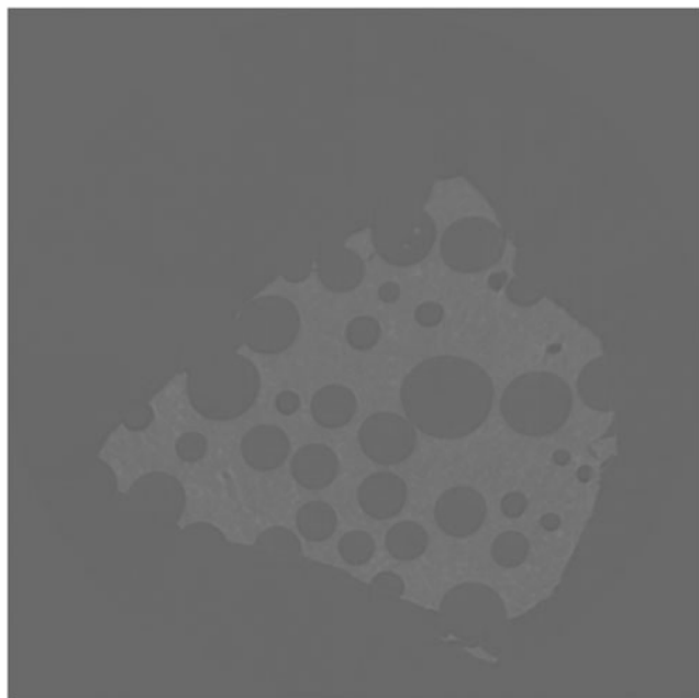
SUPPLEMENTARY FIG. S1. Raw grayscale image. The grayscale image is made into a binary black-and-white image using MATLAB's built-in graythresh algorithm, which uses Otsu's method for thresholding. The resulting image is shown in Supplementary Figure S2.
