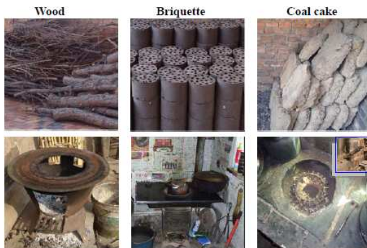
Figure S1. Pictures of the fuel and stove tested in this study. Three different fuel/stove combinations were investigated: wood burned in a simple metal stove, honmeycomb briquette burned in an improved metallic stove with a chimney, and coal cake burned in a brick stove with an outdoor flue pipe (from left to the right).
