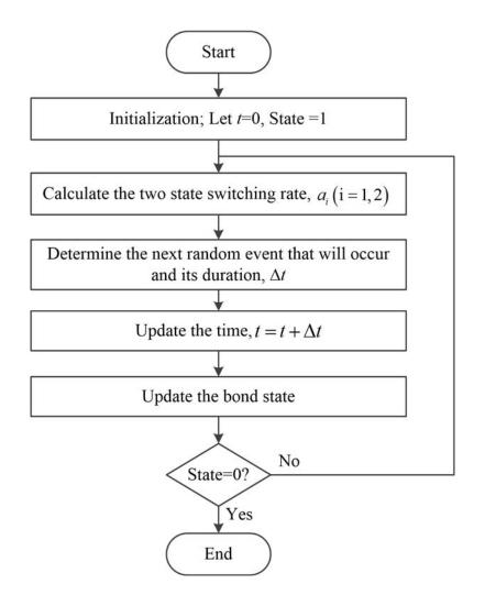
**Figure S1** Flow chart of kinetic Monte Carlo method to simulate  $T_0$  and  $T_1$  for a single catch bond.
