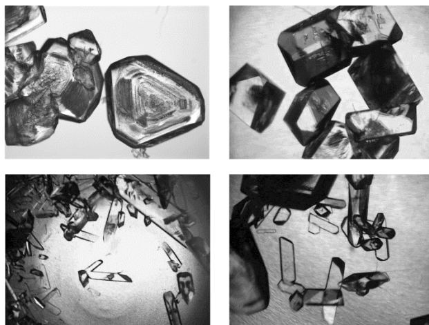
Figure S1. Morphology of acetaminophen crystals grown in the presence of p -acetamidostyrene. Clockwise from top left: no additive, 1 mM additive, 3 mM additive, and 6 mM additive.
