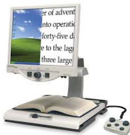
Figure 7.2. A digital camera acquires the image, which is then digitally magnified and presented on electronic display. With the widespread availability of electronic books and other media, comfortable reading on a large display becomes even more natural.
