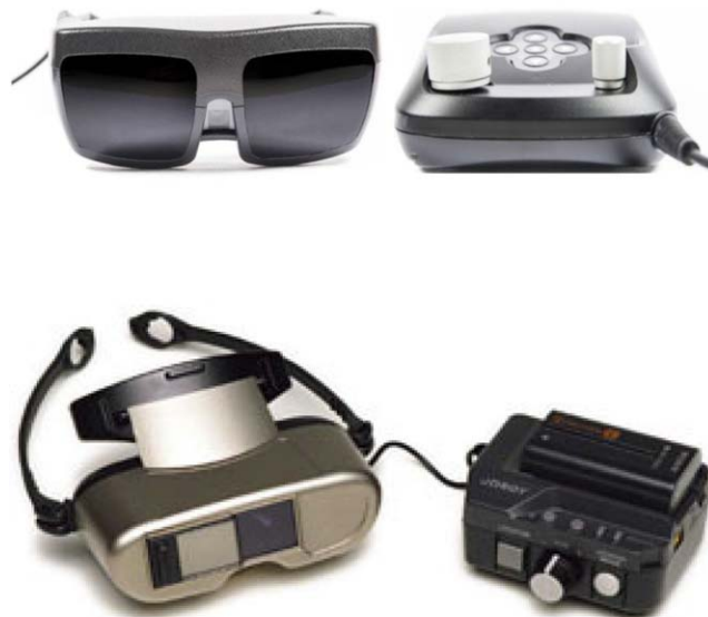
Figure 7.4. Top: Video goggles marketed by eSight. Bottom: A mobile visual aid called the “Jordy” marketed by Enhanced Vision. Both models suffer from a small field of view and cumbersome knobs to adjust parameters.
