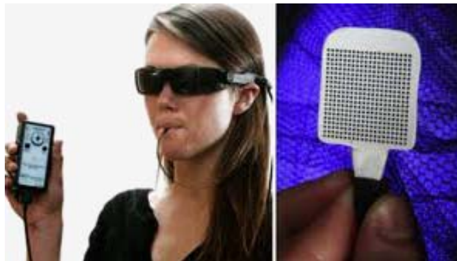
Figure 7.6. The “Brainport” generates a tactile display as an array of vibrating “pixels” placed upon the tongue. Patients have shown remarkable prowess using this device to perform sporting activities, for example. (Photo courtesy of Wicab.)
