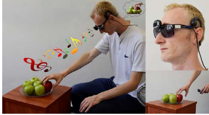
Figure 7.7. Images captured by the video camera are converted into the sequences of sounds representing brightness or color of various parts of the scene. (Photo courtesy of Amir Amedi Lab.)
