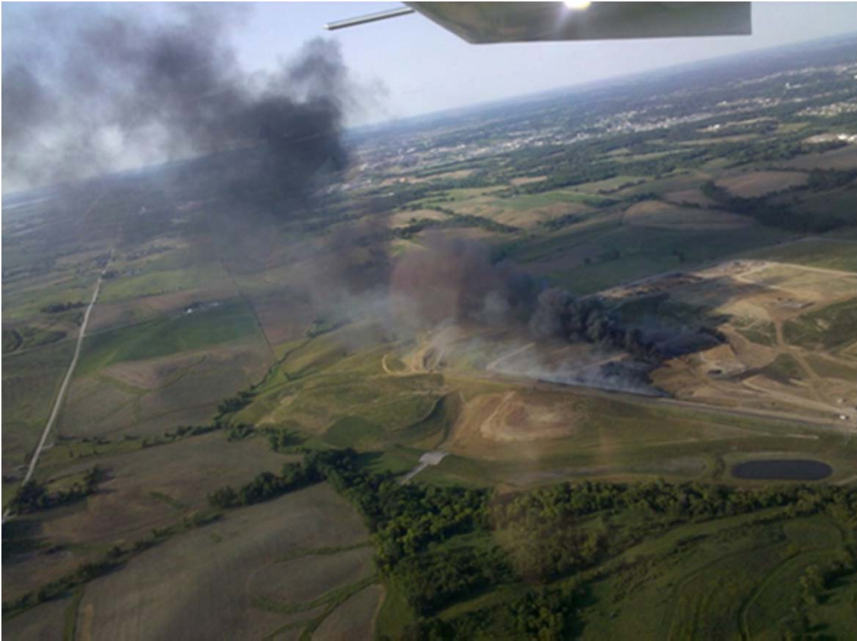
3 4 Figure 1: Photograph of the Iowa City landfill fire, with smoke primarily from the burning shredded tire 5 drainage layer 6
